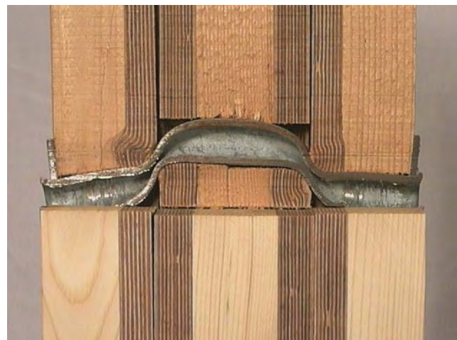
Figure 11: cut open view of the tube connection
